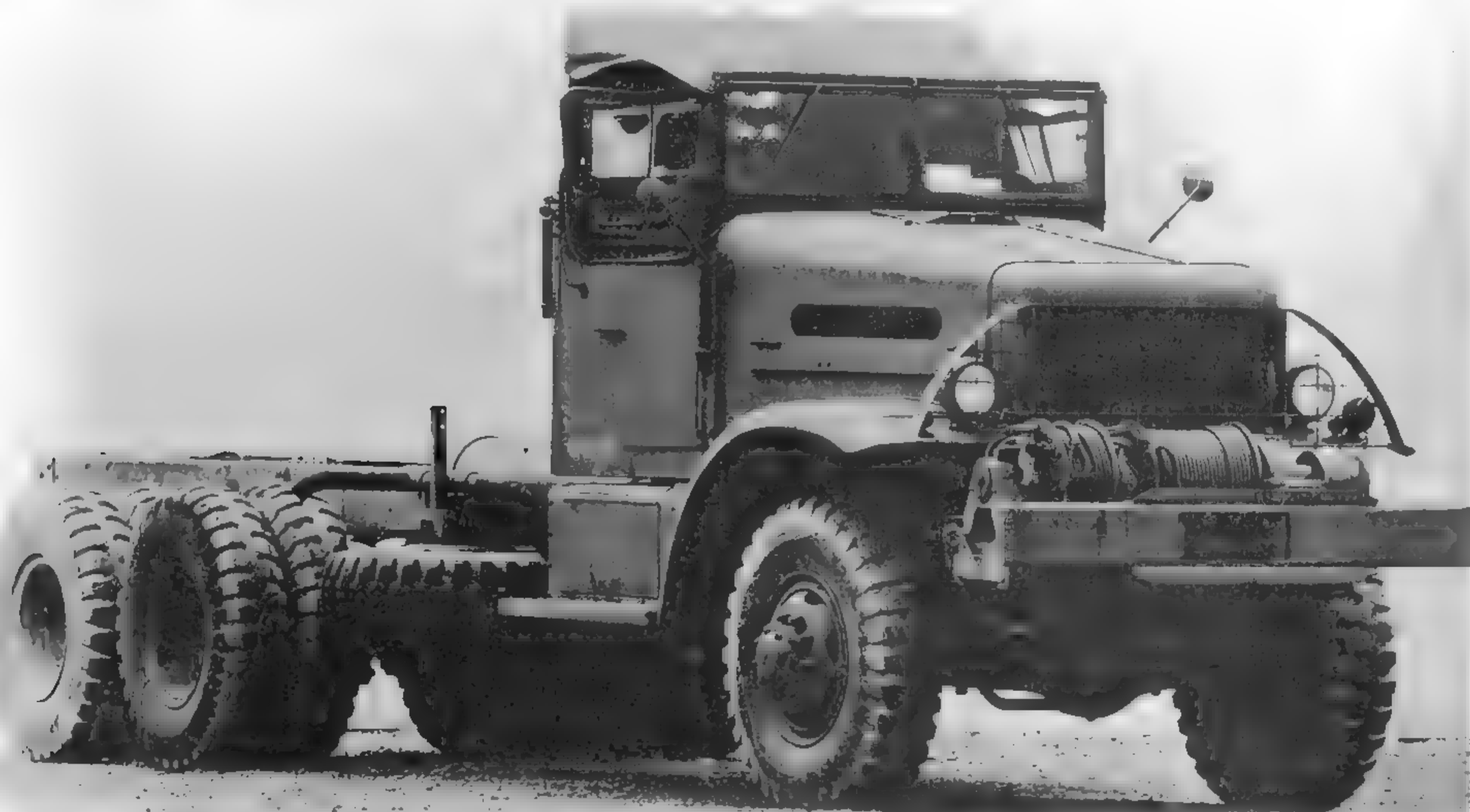
Like Corbitt, White converted to production of open-cabbed trucks, like this bridge truck chassis photographed in April of 1944 at the Studebaker Proving Ground. Like many of the bridge trucks, this truck is equipped with a 25,000-lb.-capacity dual-drum winch. (U.S. Army photo)
